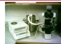
Linkam THMSG 600 heating-freezing stage at the Geofluids Research Lab.
