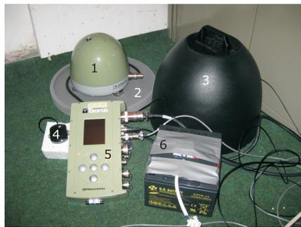
1: Trillium 120pa seismometer. 4: GPS antenna.
