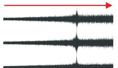
Three-component seismogram with 10 second highpass filter (periods longer than 10 seconds removed) showing 24hrs of data at IAAV on 25th October 2010. The arrow indicates the increase in wind speed and seismic wave energy during this day.
