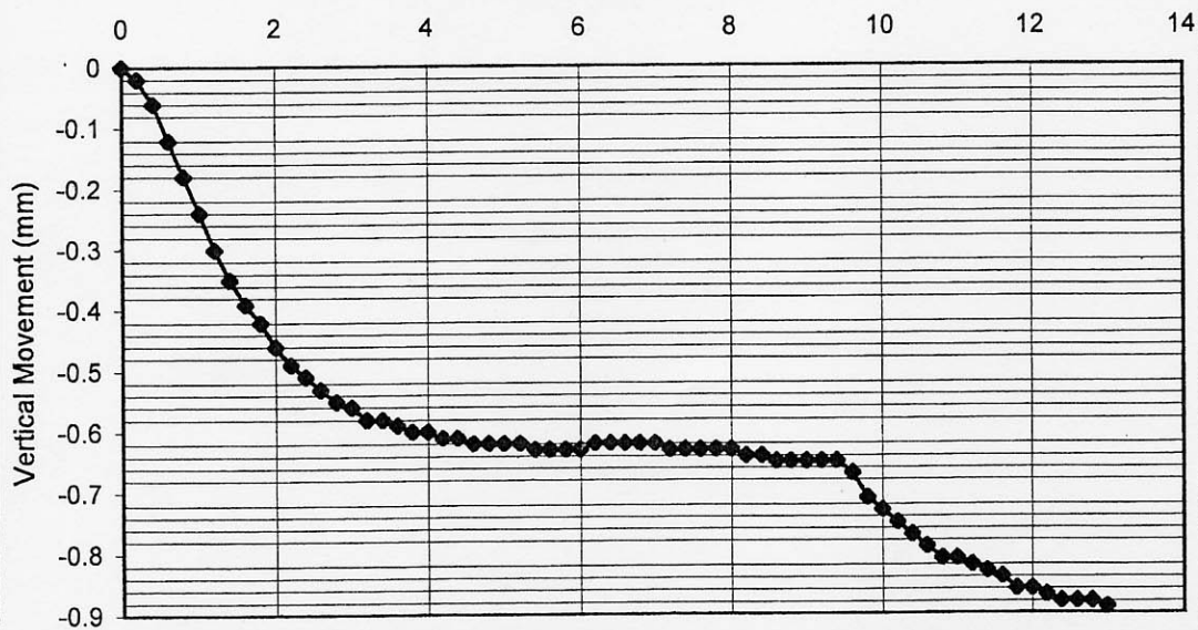
Shearbox Test No. 3 for 83/24 SC002 0.7 / 0.9 m Normal Stress 104kPa Horizontal Displacement (mm)
