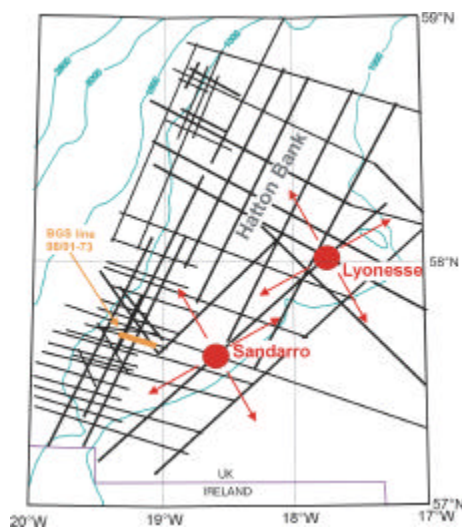
Figure 1. BGS Rockall Consortium seismic data coverage across Hatton Bank (black lines). Location of BGS line 98/01-73 is highlighted in orange. Lyonesse and Sandarro are (?Tertiary) igneous centres which have extruded lavas in a radial pattern (shown diagrammatically). Bathymetry contours in blue (depths in metres).
