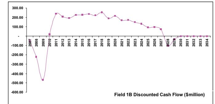
Field 1B is a dry gas field with initial gas in place of 1tcf, a recovery rate of 70% and condensate of 1bbls/mmcsf. The pipeline to shore would be routed allowing flexibility in the event of seafloor geohazards and slope instability. It is assumed booster compression will be required early in the field life to ensure adequate flow pressures.
