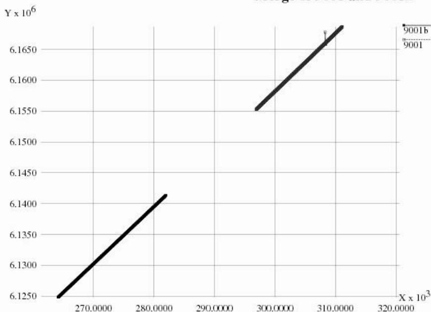
We could not merge 9001 and 9001m as there was no overlap between the lines. Infact the navigation data (see map on left) shows a gap of 600m at the supposed merge point.
