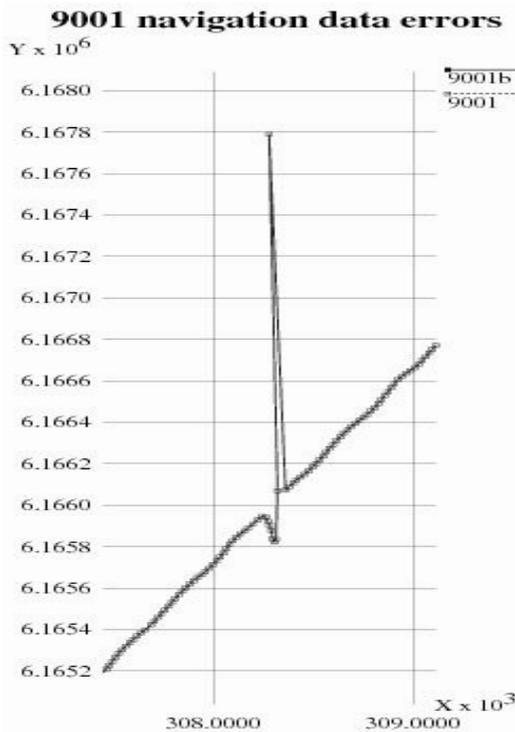
In one instance we had to interpolate a series of shotpoints 9439-9447 in order to remove spurious navigation shown in the adjacent figure.
