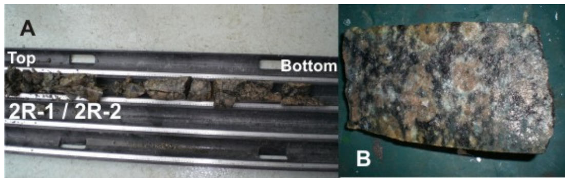
Fig. 18: About 120 cm long granite core (A) recovered at site GeoB10902. Plagioclase crystals with up to 4 cm diameter are found in this granite (B)
