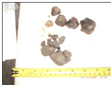
Fig. 10: Granitic gravel and mud samples found in the barrel magazine after recovery of the drill rig from deployment GeoB10901-1
