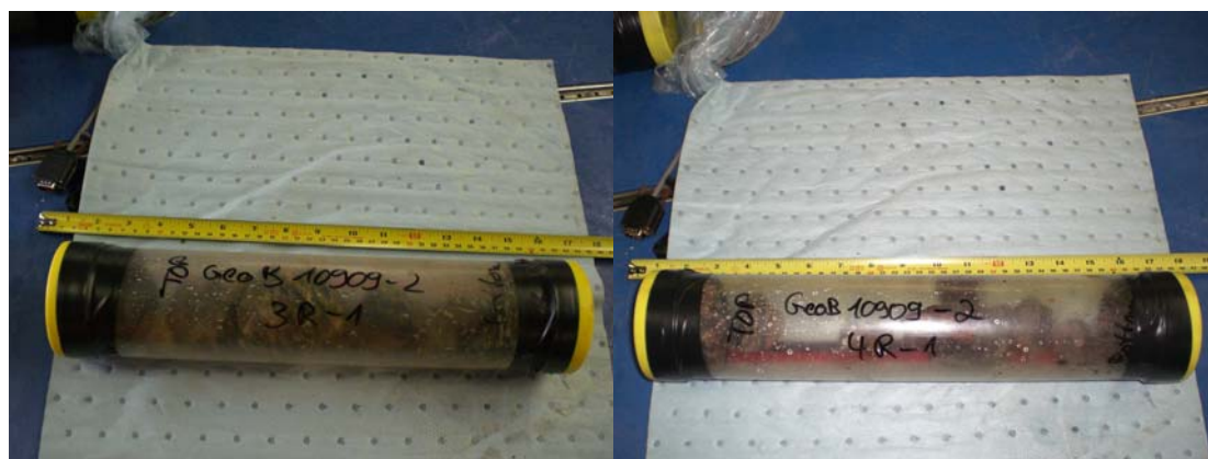
Fig. 13: Granite angular pieces from core barrels GeoB10901-2-3R-1 and GeoB10901-2-4R-1 in plastic liners
