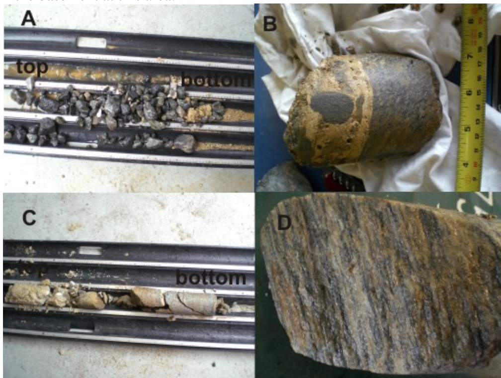
Fig. 22: Examples from the core recovery at site GeoB10903. A: subangular partly rounded metamorphic gravel (GeoB10903-3R-1); B: contact conglomerate to Gneiss boulder (GeoB10903-4R-2); C: 70 cm section of breccia with large boulder of Gneiss at the bottom (GeoB10903-4R-3); D: detail of the Gneiss (GeoB10903-4R-3)
