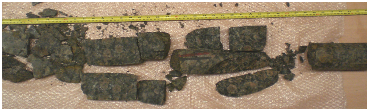
Figure 2: Photograph of K-feldspar megacrystic granulitic orthogneiss from the Porcupine High (25/7-sb (MeBo)3) showing randomly orientated K-feldspar megacrysts (pink) displaying rapakivi texture (grey rims) set in a darker matrix comprising quartz, feldspar and mafic minerals. Photograph courtesy of Mr N. Murphy, Petroleum Affairs Division.
