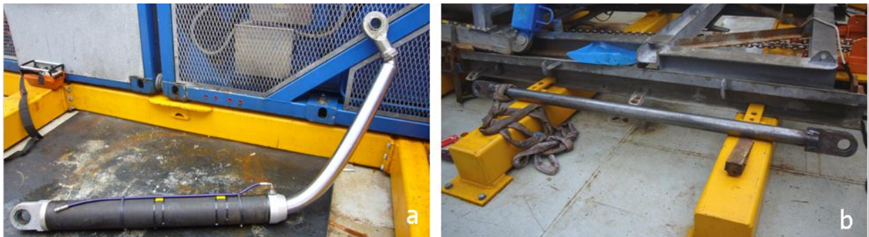
Figure 3.5: (a) Bent piston ram from MeBo leg. (b) Spare leg (photos: C. Wienberg).
