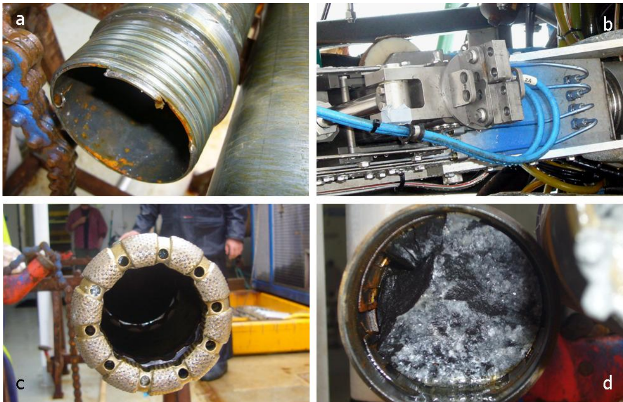
Figure 3.3: (a) Flared screw thread of outer core barrel. (b) Broken claw. (c) Diamond studded "Surface Set" drill bit for drilling limestone. (d) Limestone recovered during the first test drill (Inishmore Island, Galway Bay) (photos: C. Wienberg).
