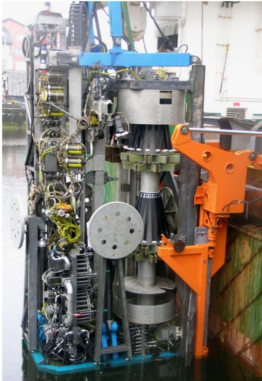
Figure 4.1: The MeBo seafloor drilling rig on the launch and recovery system over the stern of the RV Celtic Explorer in Galway Dock at the start of the cruise. Clearly visible facing the camera is one of the four hydraulic legs and circular footplate which are lowered before seabed landing, the rotary magazine into which empty and filled core barrels are stored (currently empty).
