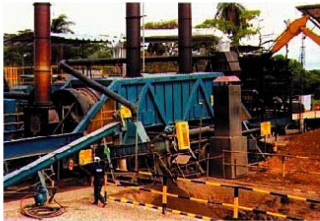
Cleaned cuttings at the BP BA-J20 site (bottom center) are being discharged from the dryer unit through the rehydration auger. The trackhoe bucket (top-right) feeds raw cuttings slurry into the feed hopper (Fig. 7; photograph by Brad Wood, courtesy of Brandt).
