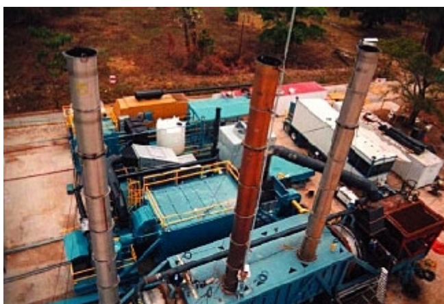
The BP BA-J20 drilling site in the Casanare area of Colombia in February 1999 during initial installation reveals (bottom to top) equipment layout for dryer, baghouse, condensers, oil-water separator, generators, and (right) control room. (Fig. 4; photograph by Douglas M. Odle, courtesy of Brandt)
