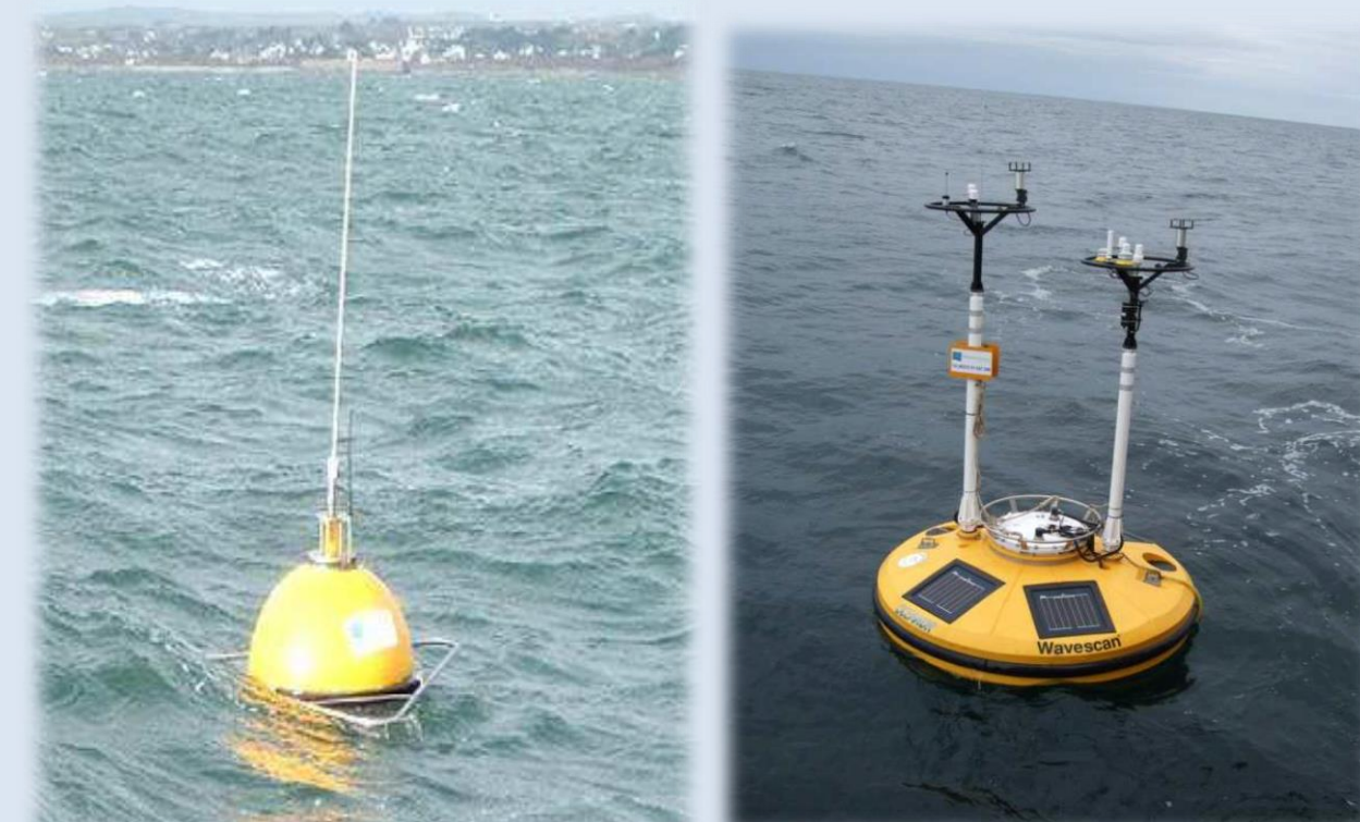
Figure 2. Datowell WaveRider and Wavescan buoys at the quarter scale test site in Galway Bay. Image courtesy of the Marine Institute and SEAI.
