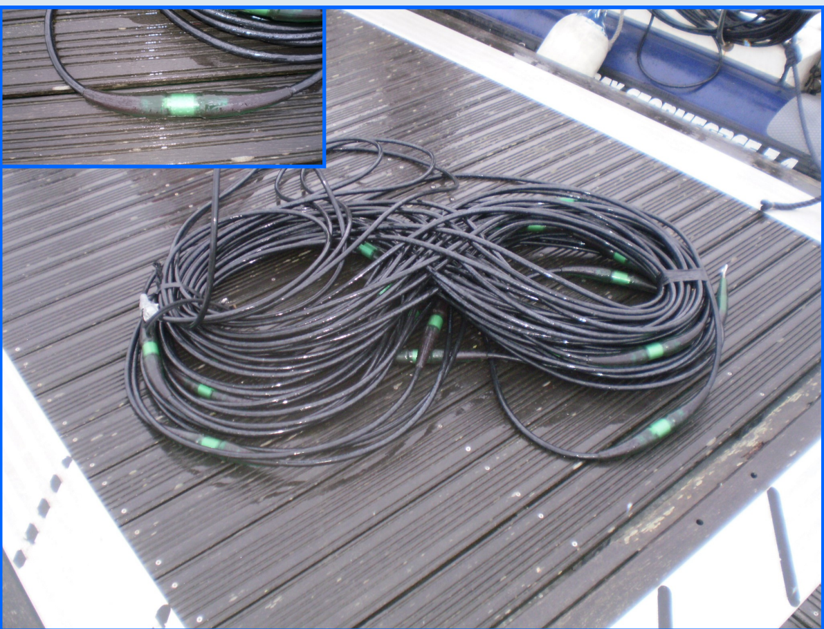
Figure 5: Geometrics DHA-7 hydrophone cable
