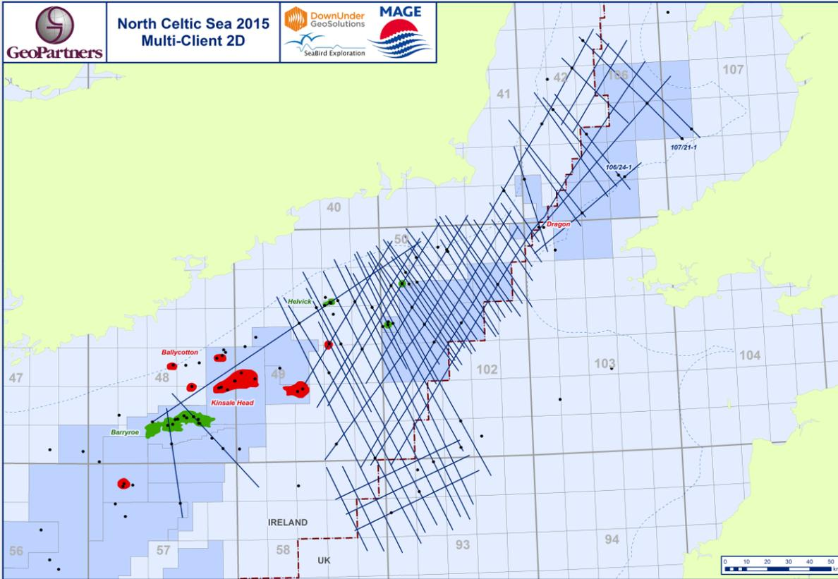
Survey acquired in summer 2015 by MAGE vessel Nikolay Trubyatinski equipped with a modern solid streamer and processed by Down Under Geosolutions in London on behalf of GeoPartners
