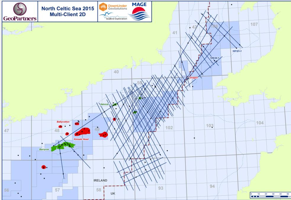
A new basin wide 2 D seismic survey has been acquired in 2015, processed in 2016 and provides a dataset with excellent shallow definition and deep penetration that allows the regional evaluation of both plays and basin development, putting exploration targets in context.
