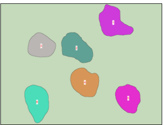
Fig. 3 (c) Individual grain regions identified using Watershed Transform algorithm.
